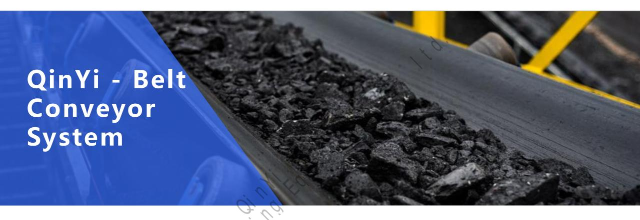
It can handle all kinds of powders, granular and bulk materials in a continuous material flow from the loading point to the unloading point on a certain transportation line. It not only plays an important role in the internal transportation of industrial enterprises, but also plays an important role in its external transportation.
