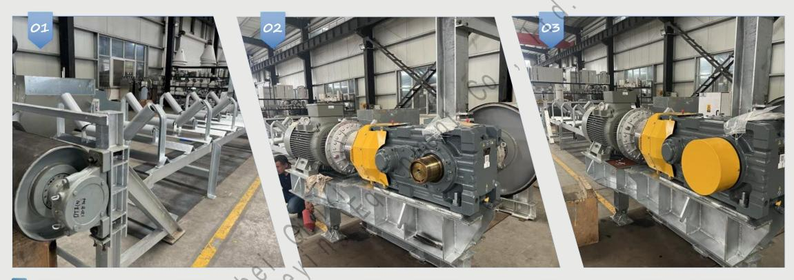
Belt conveyor is a category of continuous conveying machinery. It is a continuous conveying equipment that takes the conveyor belt as the traction component and support component, uses idler to support and relies on the friction force between the driving pulley and the conveyor belt to transfer the traction force.
